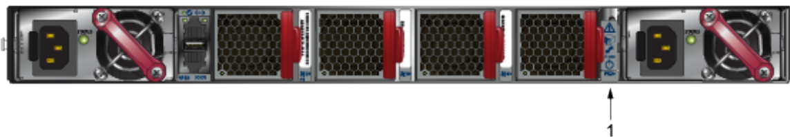
Figure 15: Earth Grounding Pad Sockets for Models with Management Ports on the Rear Panel
