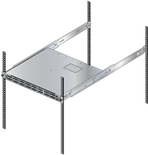
Figure 13: Attaching the Switch to the Rack Posts
