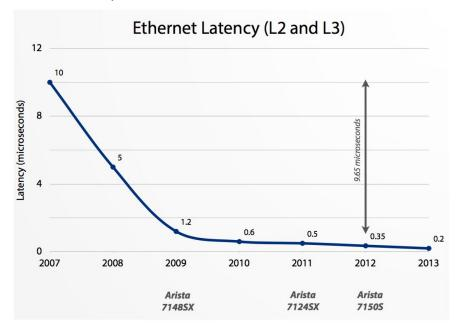
Figure 1 shows how cut-through forwarding has decreased the latency bar for highdensity 10G switches. Starting in 2009, where a regular switch might introduce 10us per hop, Arista Networks 7148SX reduced this to 1.2us – an 88% reduction for 48 x 10GbE solutions.
