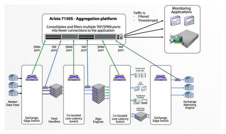
Figure 10: Common platform for Advanced Mirroring and TAP Aggregation
