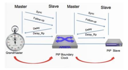
As an example, if a master clock is capable of supporting 100 devices, and each boundary clock can support an additional 100 devices, the PTP implementation can scale by 100X by implementing a single tier of boundary clocks in the network,
