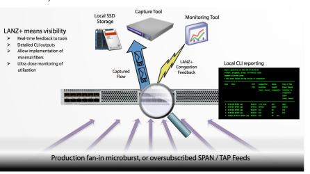
For forensic purposes, LANZ+ is able to capture a sample of the packets that were queued in a congestion event. This provides application level latency performance monitoring from all angles – always-on proactive, triggered reactive, flow- based, and real time packet sampling.
