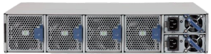
Arista 7250QX 2RU Rear View: Rear-to-front airflow model
