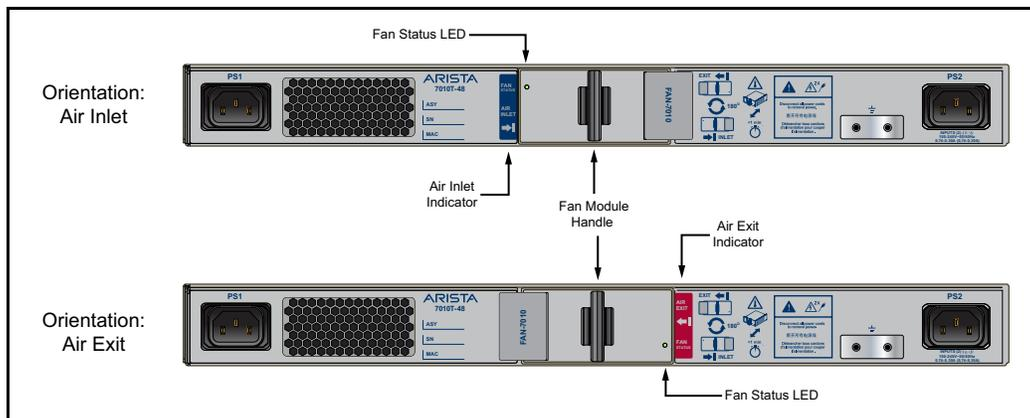
**Figure 1: Rear Panels with Contrasting Fan Module Orientation**
