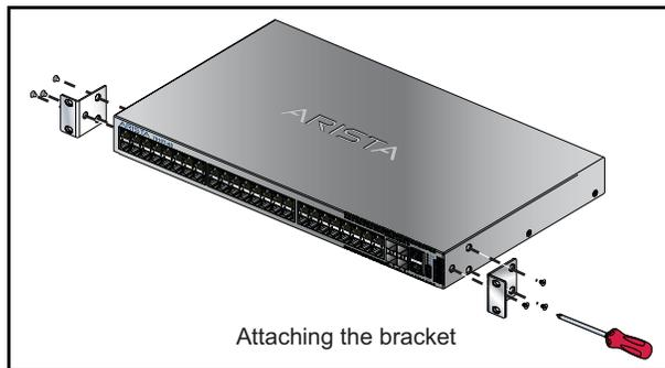
**Figure 3: Attaching the Mounting Brackets to the Switch Chassis**
