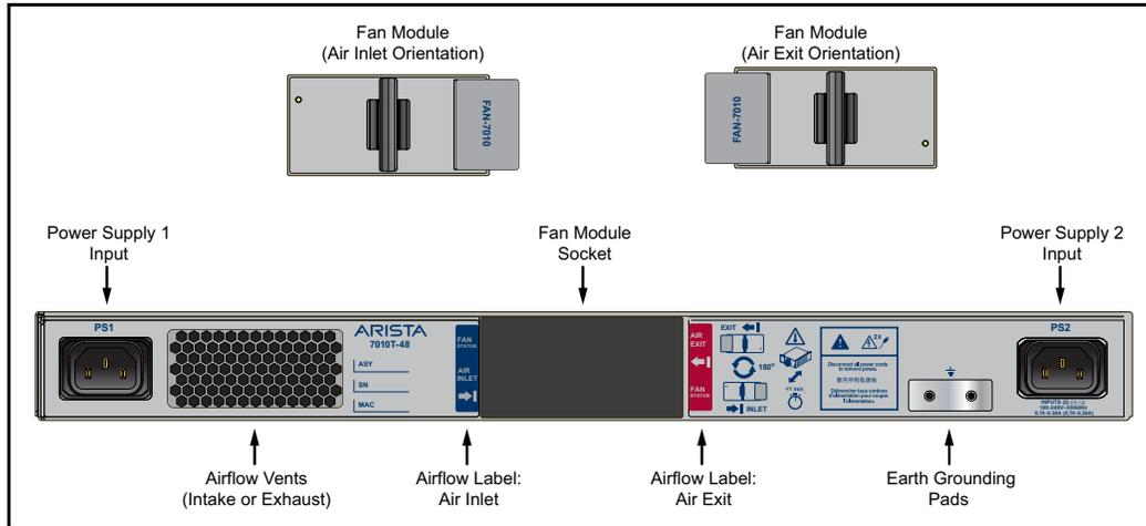
**Figure 10: Orienting the Fan Module**
