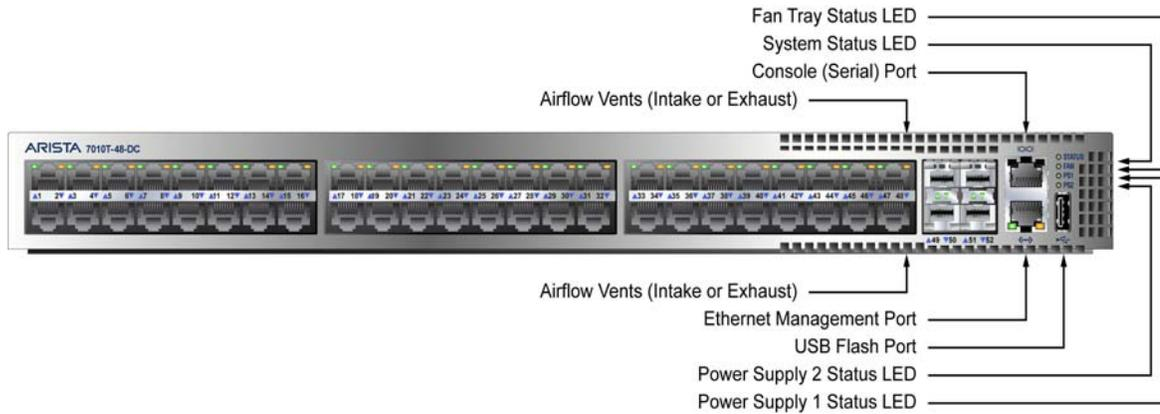
Figure 17: DCS-7010T-48-DC Front Panel
