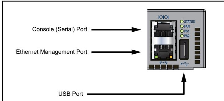
**Figure 9: Front Panel Ports**
