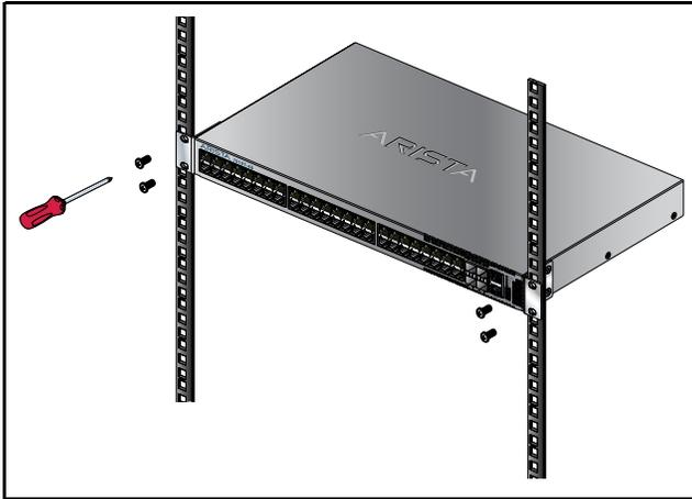
**Figure 4: Inserting the Switch into the Rack**
