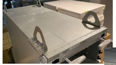
Lifting brackets and mounting hardware included in accessory kit shipped with chassis
