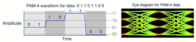
When a signal is referred to as "25Gb/s NRZ" or "25G NRZ", it means the signal is carrying data at 25 Gbit / second with NRZ modulation. When a signal is referred to as "50G PAM-4", it means the signal is carrying data at a rate of 50 Gbit / second using PAM-4 modulation.
