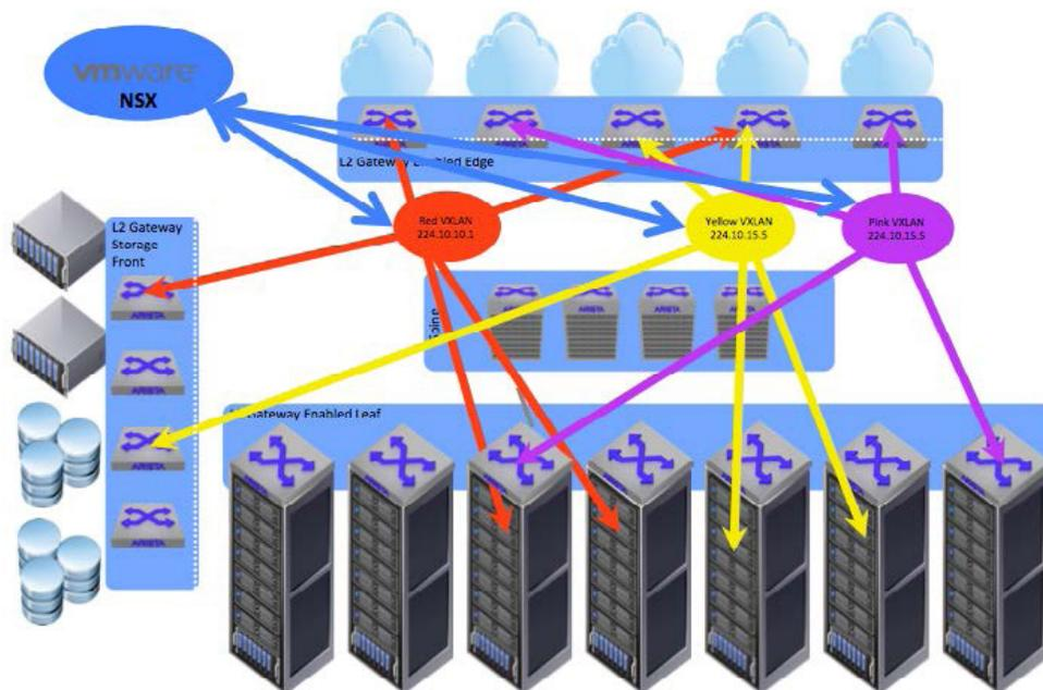
NSX's L2 Gateway programmability across both VMware and Open V-Switch Data Base (OVSDB)-server environments seamlessly integrates with Arista's hardware-based VXLAN implementation to bridge these logical networks across multi-vendor virtual server environments and physical infrastructure gateways.
