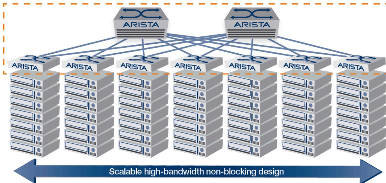
This two-tiered Leaf-Spine architecture allows connections scaling to 50,000+ end user ports nodes providing maximum throughput for your data sets. At the spine, routing between the leaf switches that have the highest traffic exchange is desired. At the leaf, line rate performance enabling scale-out application deployments is highly desirable. This scaled out high bandwidth design allows for optimizing the performance of a job by minimizing ingestion/egestion and RPC retransmissions.
