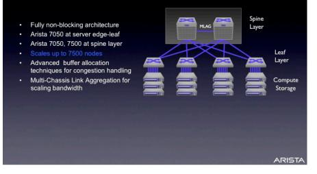
available then a layer-3 design is recommended. To insure maximum flexibility Ethernet switches should provide both layer 2 and layer 3 forwarding options.
