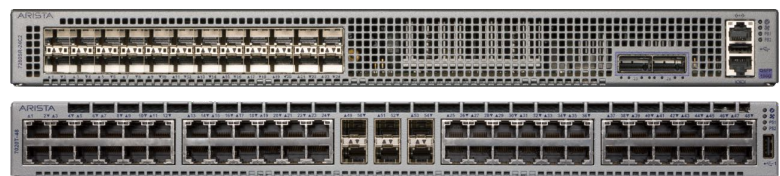
7020R: 24 port 10G and 48 port 100/1000 Mb and 6 port 10GbE Switch
