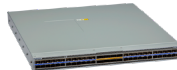
Arista 7050SPX4-48D8: 48x 100G DSFP ports, 8x 400G QSFP-DD
