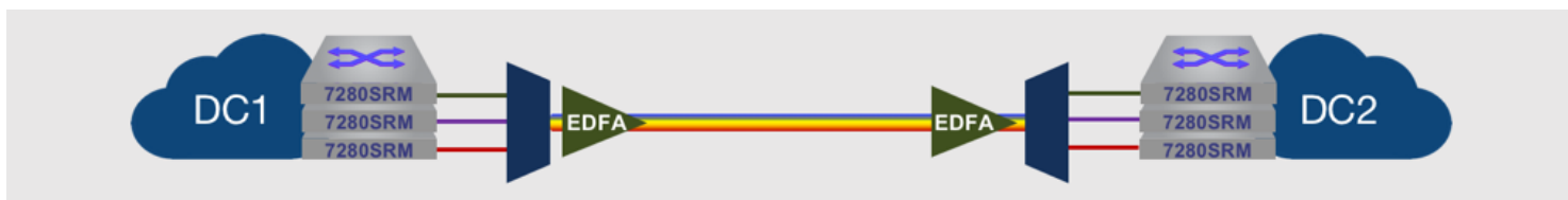
Figure 2: Amplified metro / long-haul DCI (500km - 2500km+ depending on modulation)
