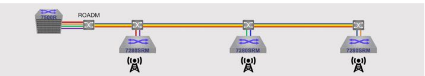
Figure 4: Mobile back-haul and metro aggregation
