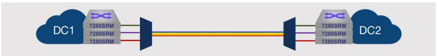
Figure 1: Un-amplified metro DCI (80km - 100km)
