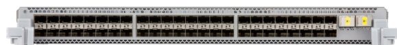
48 port SFP+ for 1/10GbE and 2 port 100GbE SR10 MXP line card - Up to 72 10G ports per line card or 48 1/10GbE ports and flexible 40G/100G - Two MXP ports allow choice of 2 x 100GbE, 6 x 40GbE or 24 x 10GbE
