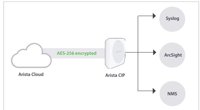
installing and maintaining an on-premise Arista Wi-Fi server. A Cloud Integration Point (CIP) is an Arista AP that enables the integration of the Arista Wi-Fi cloud server with existing third-party services on-premises.
