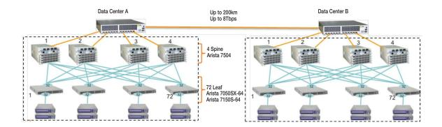
For enabling extended reach Ethernet connectivity between data centers, the Infinera CX provides the industry's most compact and power-efficient Wavelength Division Multiplexing [WDM] solution:
