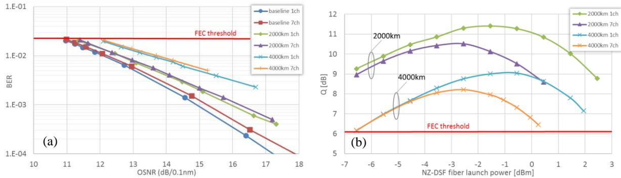
Figure 3. (a) BER vs OSNR results, (b) Launch power optimization
