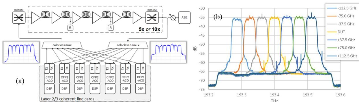
Figure 1. (a) System configuration, (b) Spectrum for 7x 32 GBaud Nyquist (RRC=0.2) PM-QPSK signals at 37.5 GHz spacing
