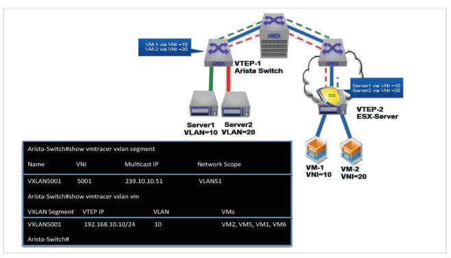
Figure 34. VM Tracer for VXLAN visibility exposes VMs and VXLAN information in VXLAN enabled network
