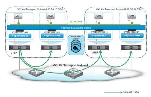
Figure 22. Unicast Mode Logical Switch
