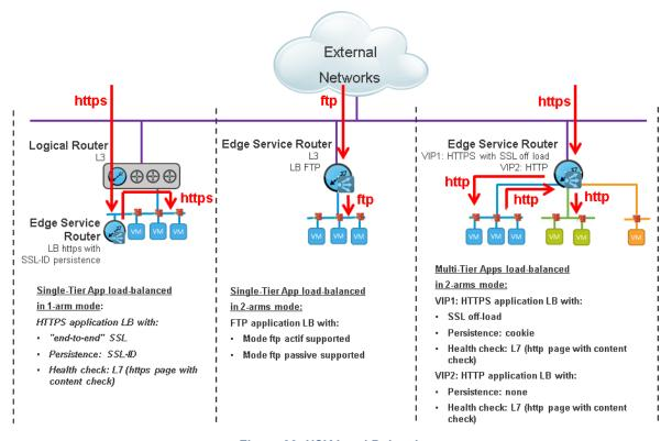
Figure 33. NSX Load Balancing
