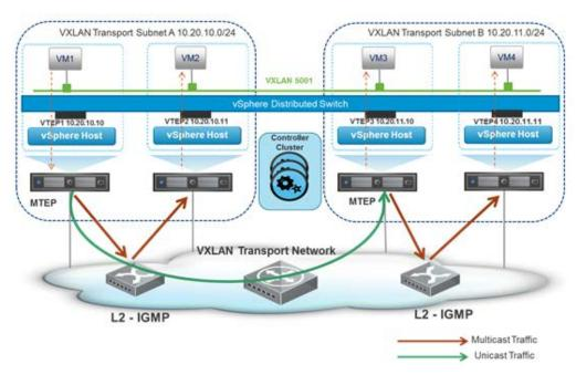
Figure 24. Hybrid Mode Logical Switch
