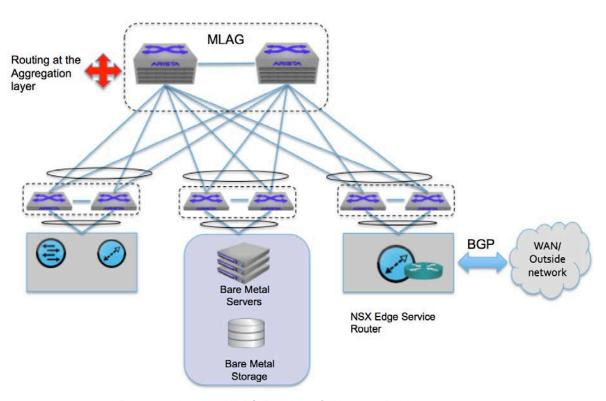
Figure 12. Layer 2 MLAG Topology for Layer 2 Design
