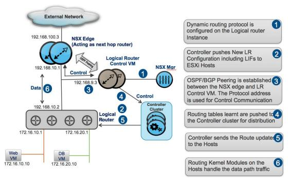
Figure 27. Logical Routing Components
