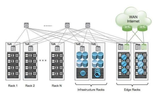
Figure 28. Logical Routing Components in the Racks
