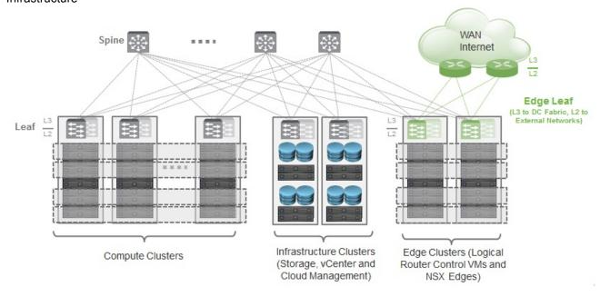
Figure 13. Data Center Design - layer-3 in Access Layer
