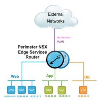
Figure 25. NAT and DHCP Configuration on NSX Edge Service Router
