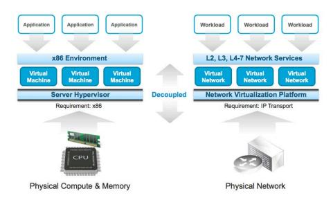
Figure 1. Server and Network Virtualization Analogy
