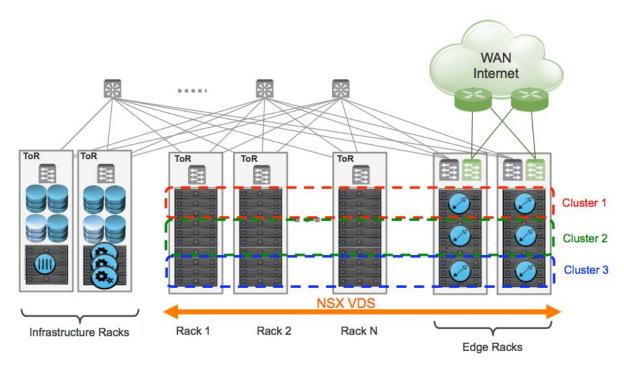
Figure 21. Logical Switching Components in the racks
