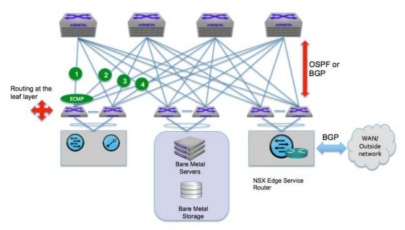
Figure 8. Open Standard Based Layer-3 leaf-spine for Horizontal Scale
