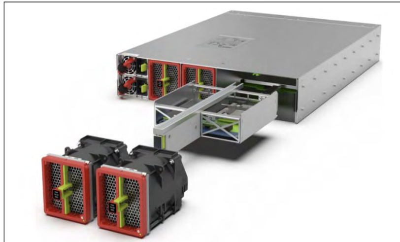
Figure 6: Removable Supervisor module on the 7060X6-64PE
