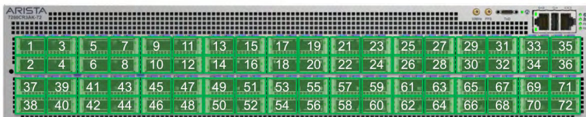
Figure 19b: 7280CR3A-72 port numbering
