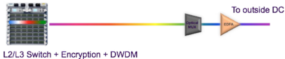
Figure 5. Arista Integrated DWDM solution with encryption
