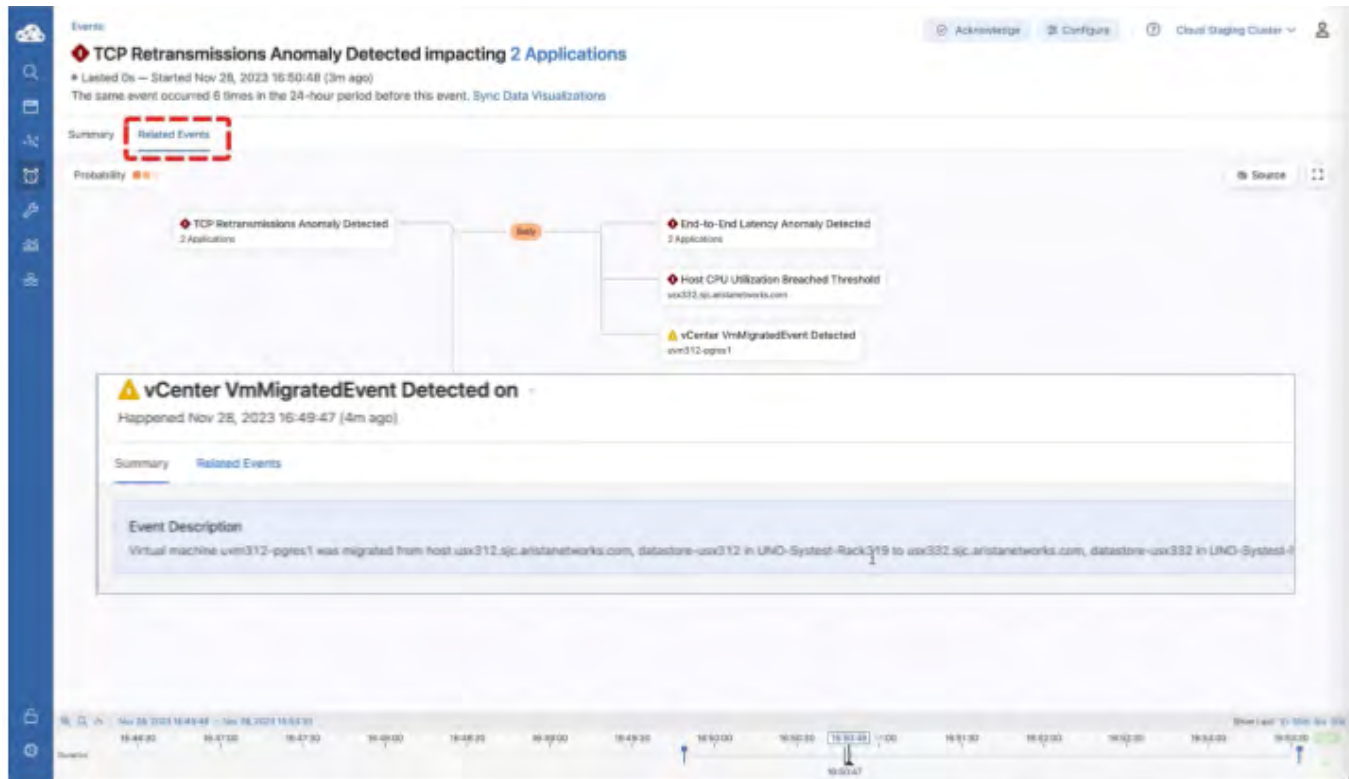
Figure 5: Using traffic analysis, AVA can provide rapid issue inference for network / application related issues
