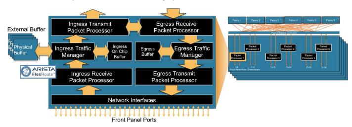
Figure 15: Packet forwarding pipeline stages inside a packet processor on an Arista~7500R~line~card~module
