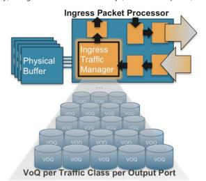
Figure 21: Physical Buffer on Ingress allocated as Virtual Output Queues
