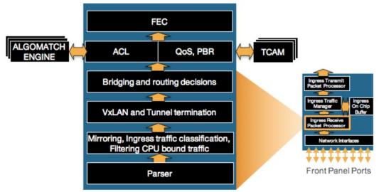
Figure 19: Ingress Receive Packet Processor with AlgoMatch
