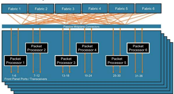
Figure 4: Distributed Forwarding within an Arista 7500R Series
