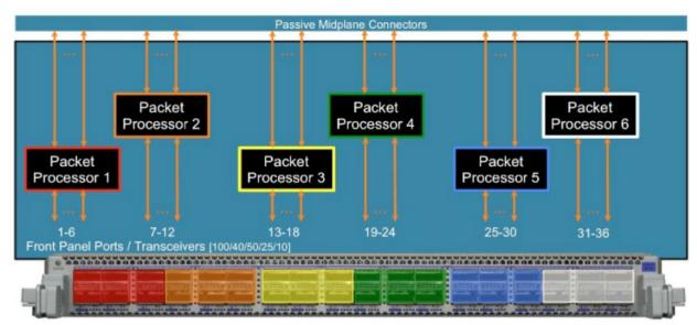
Figure 6: Arista DCS-7500R-36CQ-LC module architecture
