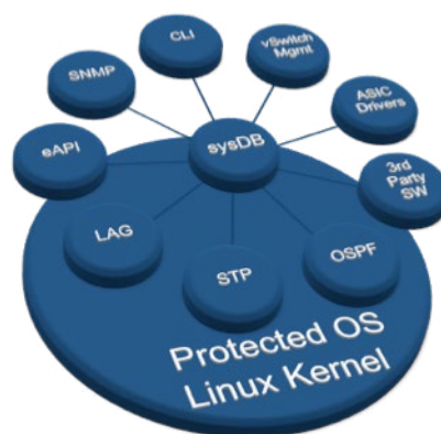
Figure 14: Arista EOS Software Architecture showing some of the Agents
