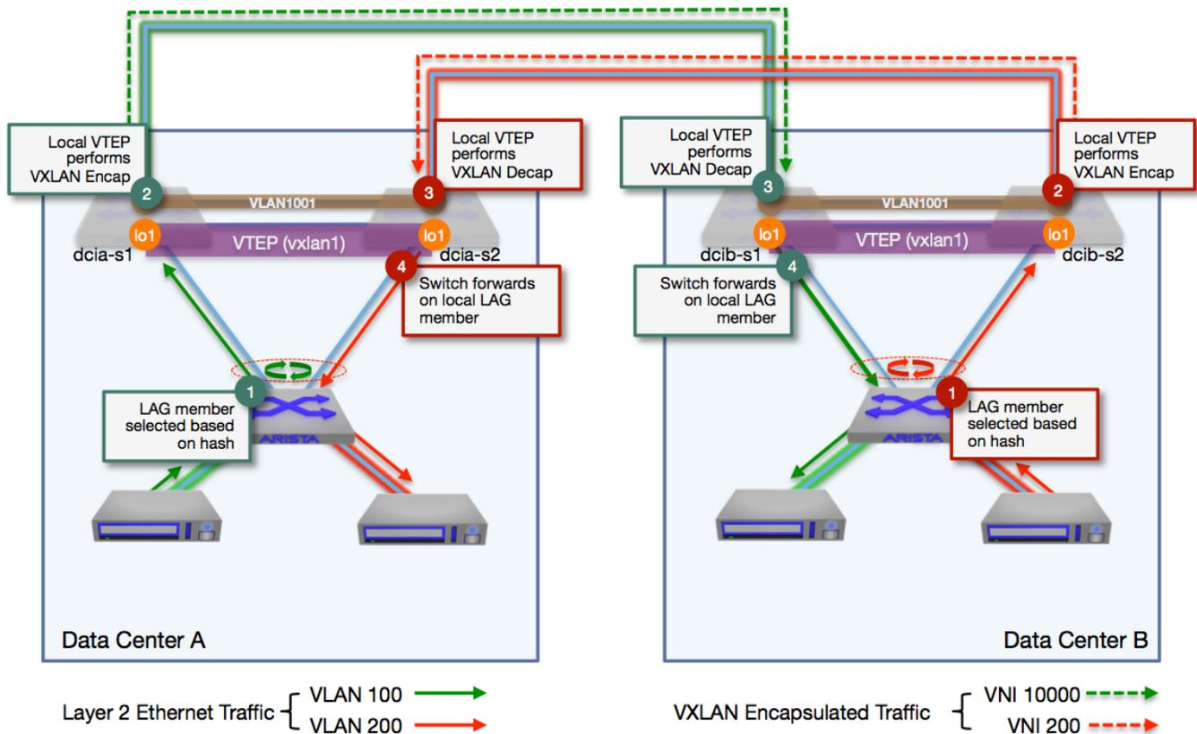
Figure 14: Normal VXLAN+MLAG forwarding Mechanism
