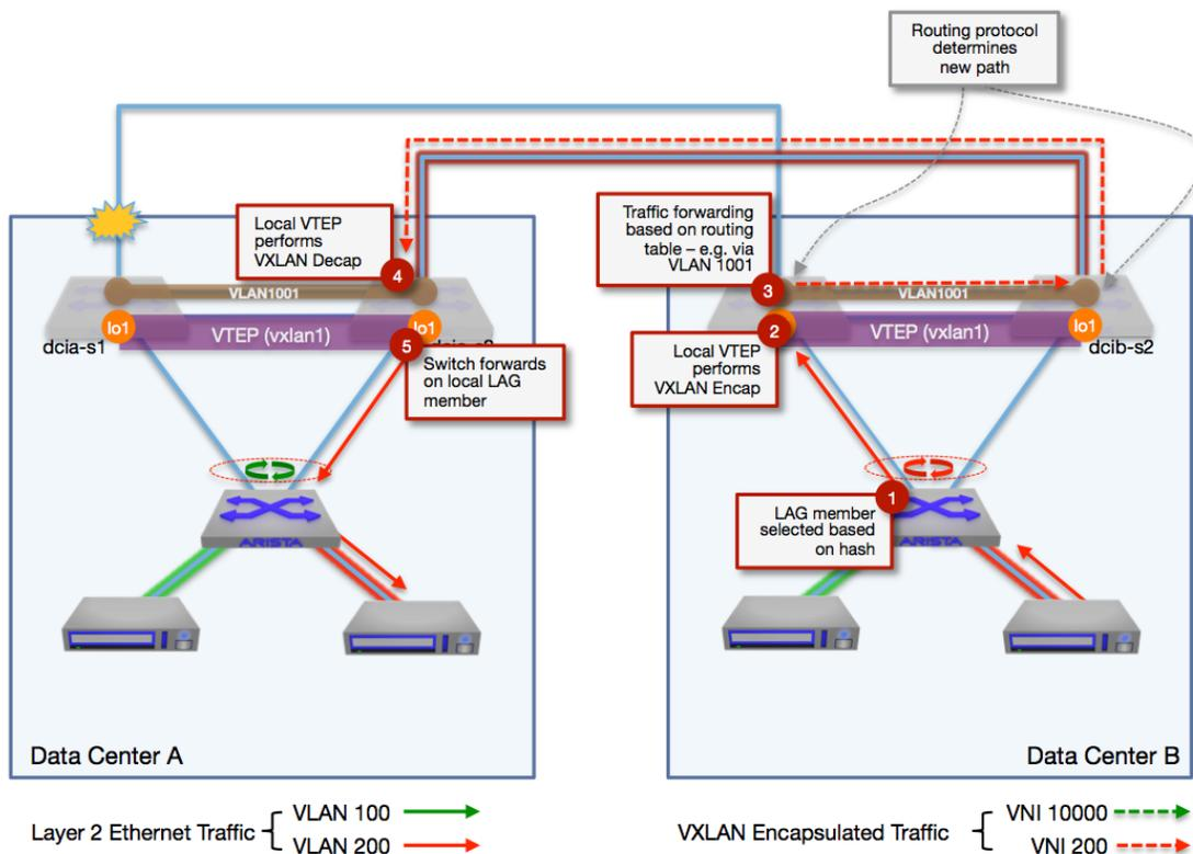
**Figure 18:** Effect of Remote DCI Inter-Site Link Failure
