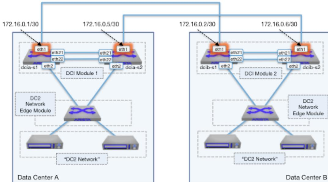
**Figure 11:** Example DCI Solution – Layer-3 Interfaces
