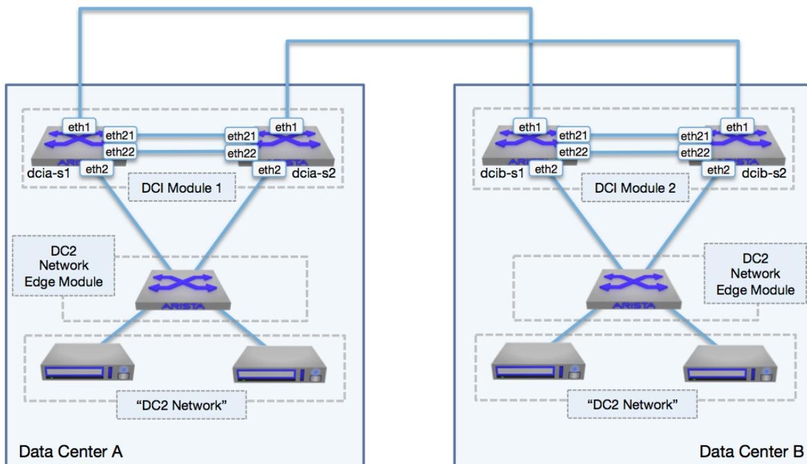
Figure 10: Example DCI Solution – Physical Topology
