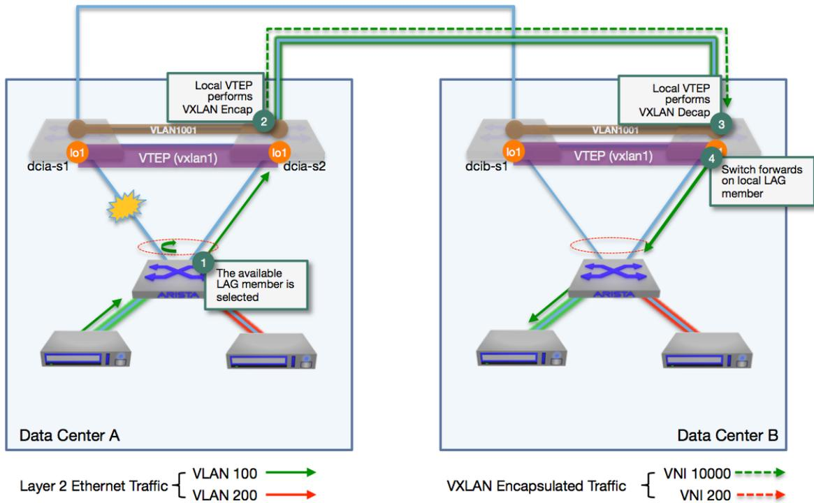
**Figure 15:** Effect of Local MLAG Member Port Failure
