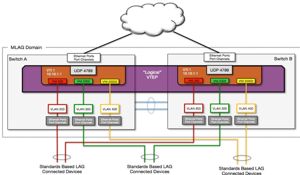
Figure 7: Arista VXLAN+MLAG Hardware VTEP Architecture
