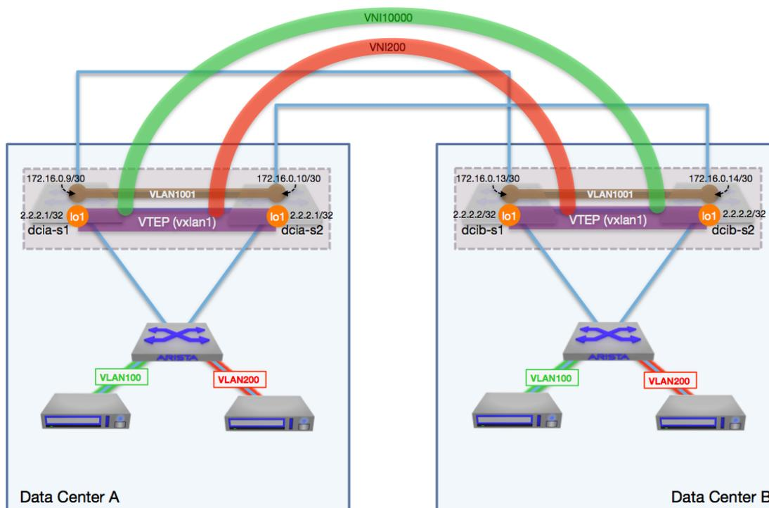
Figure 13: Example DCI Solution – VLAN & VXLAN Topology
