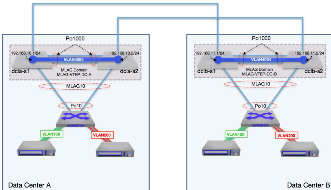
Figure 12: Example DCI Solution – MLAG Topology
