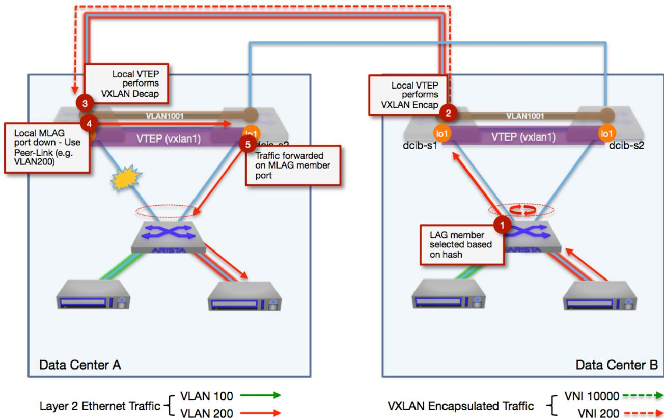
Figure 16: Effect of Remote MLAG Member Port Failure
