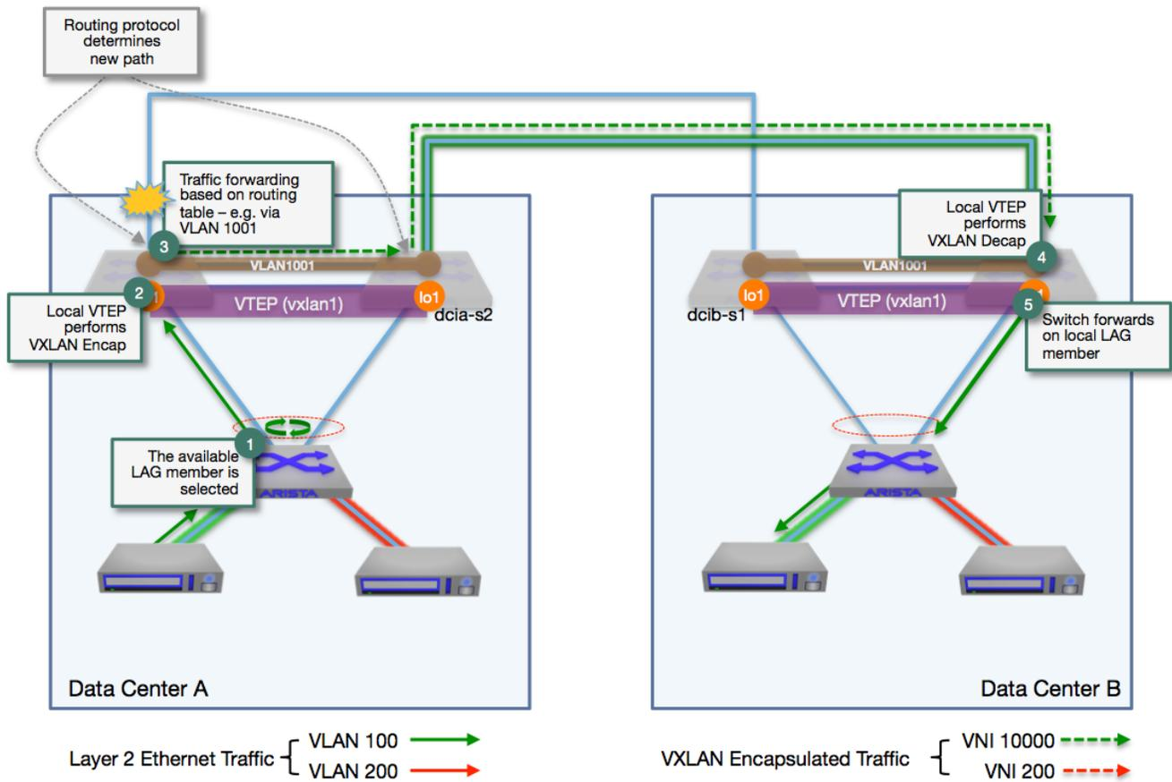
**Figure 17: Effect of Local DCI Inter-site Link Failure**
