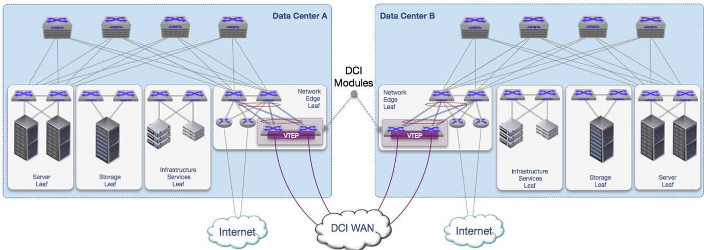
**Figure 9:** Integration of the DCI module with a Leaf-Spine Data Center Network
