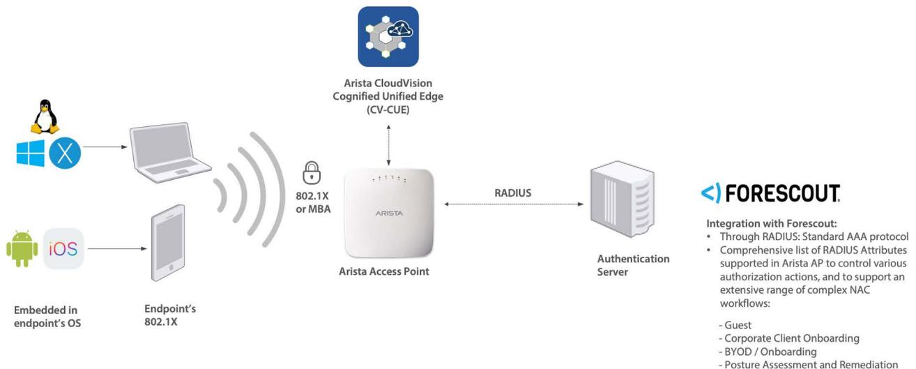
An Arista access point (AP) supports Wi-Fi client authentication using 802.1X or MAC-Based Authentication (MBA) and exchanges RADIUS messages with Forescout. The following workflows are supported:
