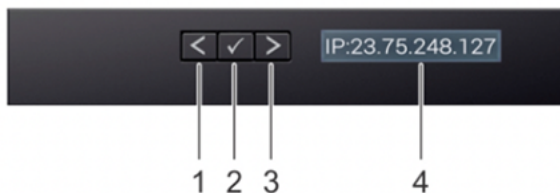
Figure A-1: LCD Panel Features
