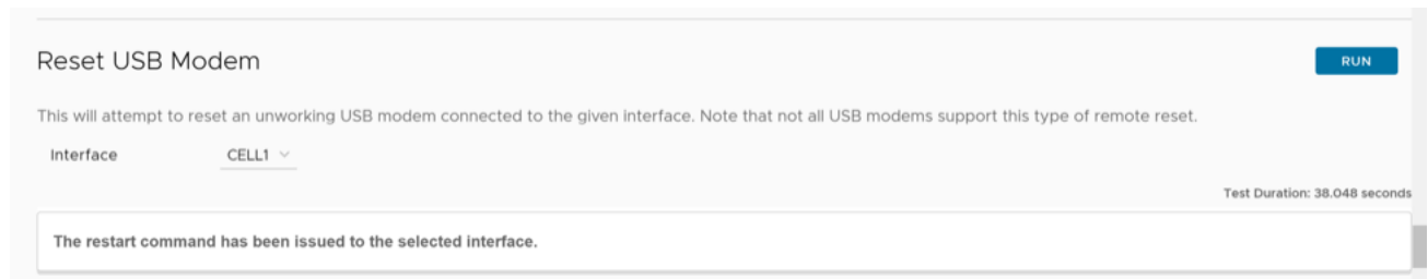
Figure 5-76: Running a Reset USB Modem Test
