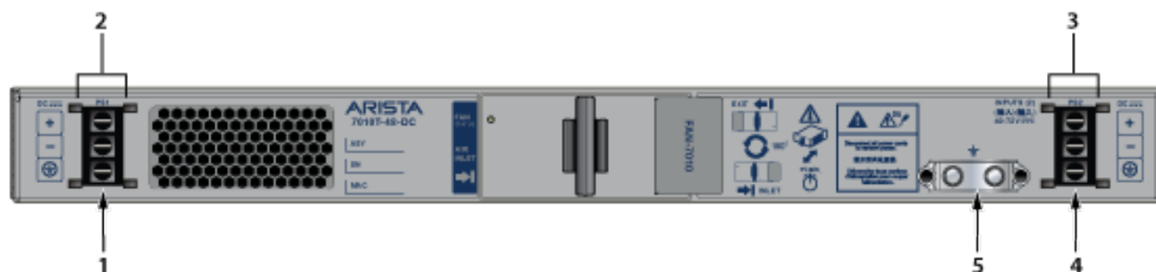
Figure 4-2: Grounding Points and Power Terminals for 7010T-48-DC and 7010TX-48-DC Switches
