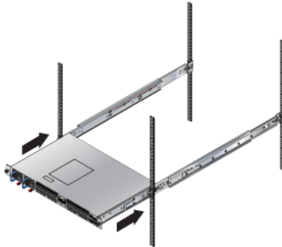
Figure 3-6: Inserting the Switch onto the Rails
