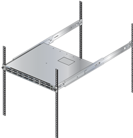
Figure 3-12: Attaching the Switch to the Rack Posts
