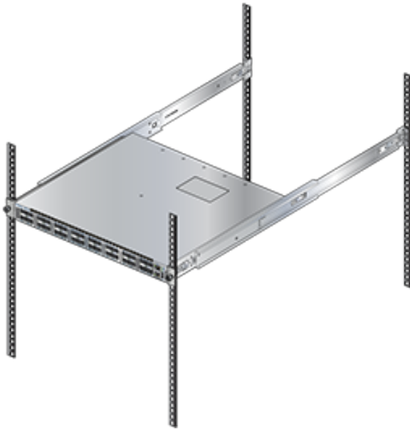
Figure 3-12: Attaching the Switch to the Rack Posts
