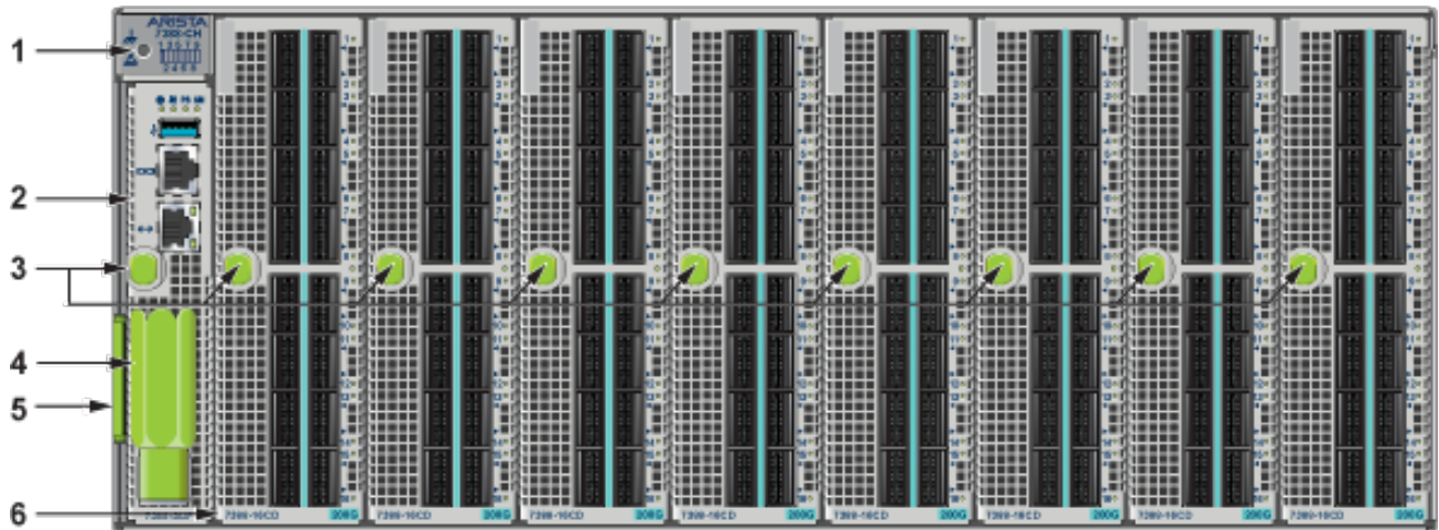
Figure C-1: DCS-7388X5 Front Panel (fully populated)
