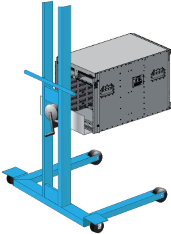
3. Secure the chassis by tightening the thumbscrews on the front flanges into the rack posts, as shown in the following figure.
