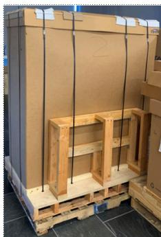
1. Cut away the straps and remove the cardboard to expose the chassis with the rack kit basket attached and nested on top of the chassis.
