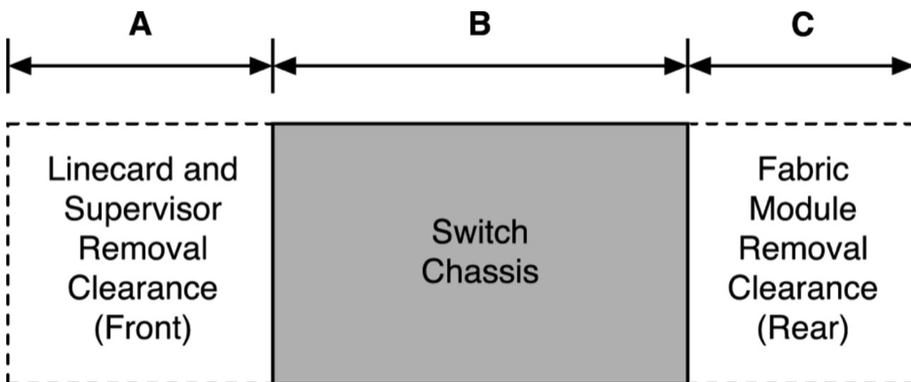
The [Figure 2-1: Clearance Requirements and Footprint for Switches](#) display the dimensions and footprint of the switch clearance requirements.
