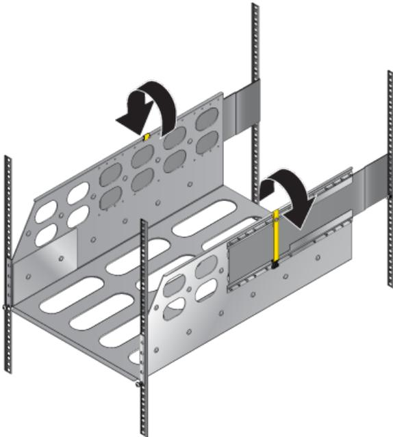
7. Secure the cradle to the rack posts using the eight remaining screws, two more in the front and six more in the back, for a total of twelve screws.
