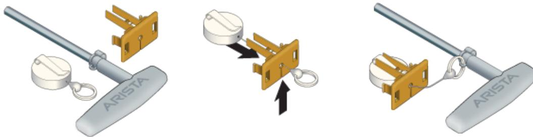
Use the following steps to attach the tethering mechanism to the extraction tool.
