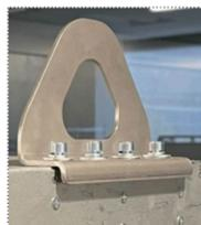
3. Attach the 1000 lb lifting straps to the lifting brackets on the chassis and the loops through the prongs of the lift.
