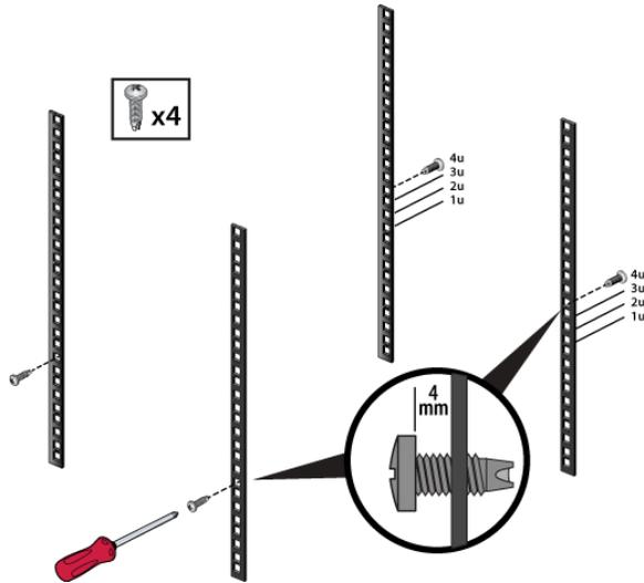
**Figure 3-3: Mounting (Starting Screws) Locations for Cradle (Front and Rear)**
