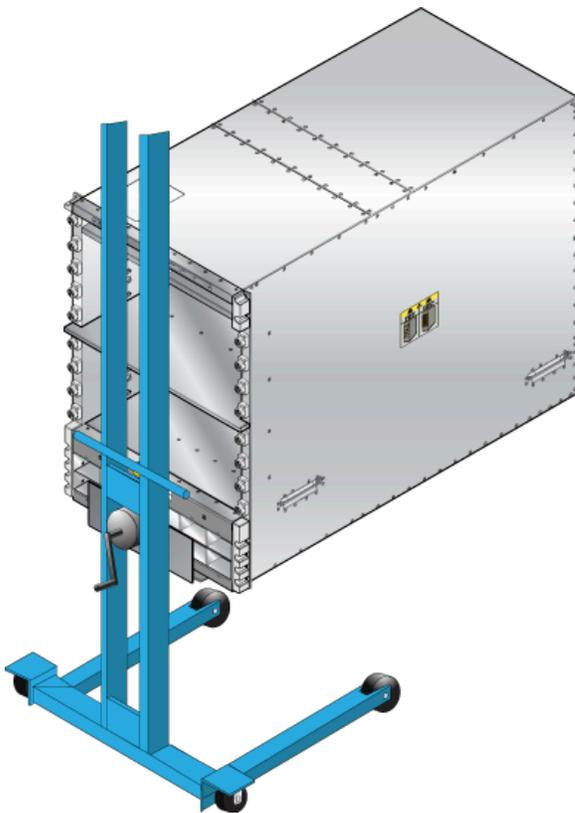
3. Secure the chassis by tightening additional M6 screws on the front flanges into the rack posts.
