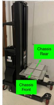
5. Align and move the chassis into the rack using the translatable platen.
