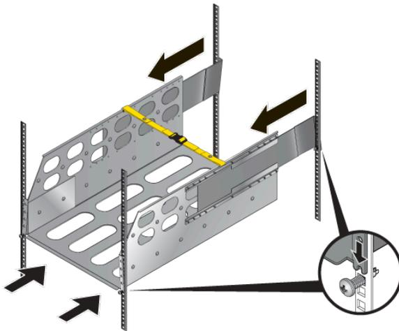
6. Release the clasp on the connector to rotate the left and right sides so they are vertical.
