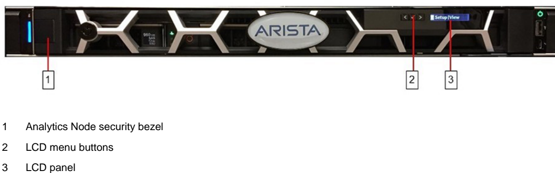
Figure 3-2: Arista Analytics Node (DCA-DM-AA3) Front Panel
