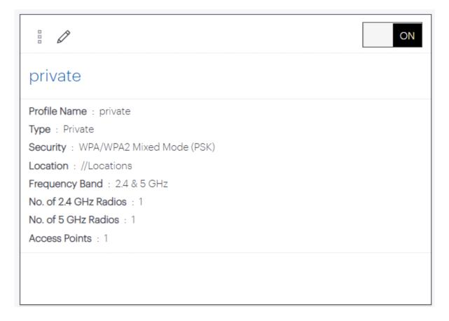
3)Confirm the encryption standard configured for the 2.4GHz SSID(s):
