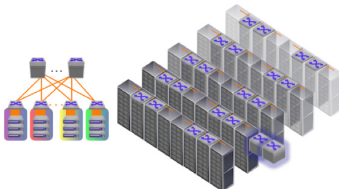
Figure 2: Arista Spine/Leaf two-tier network designs provide scale in excess of 100,000 physical servers
